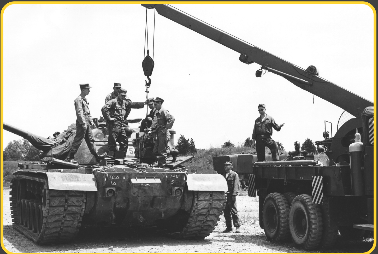
Personnel of the 357th Ordnance Company prepare to change a "Little Joe" engine on a M48A1 tank during annual training in 1959.
